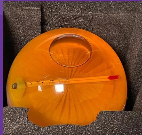
Issue with internal thermometer which stopped working therefore new customised design introduced
