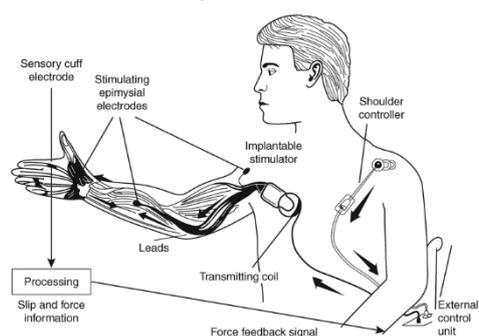
Fig. 1 Overview of the NeuroControl FREEHAND<sup>®</sup> system
